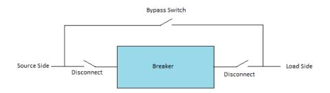
Figure 12: Example of Bypass Switch Installation
